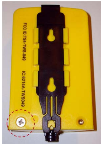
Figure 1 - Remove Screws on Back of Sensor
