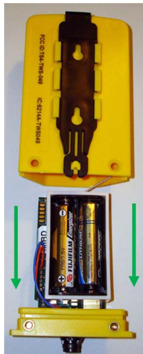
Figure 2 - Gently Remove Base by Pulling Down
