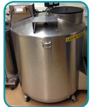
*Liquid Nitrogen Tank – has a 418MHz wireless temperature transmitter and RTD Cryo Probe installed to monitor temperature inside the tank*
