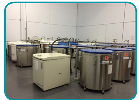
Liquid nitrogen tank storage room
